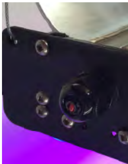
Gland-Nut Provides access to 0-10V Dim Control
