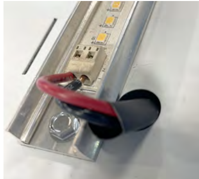
Using heat-shrink tubing to protect the LED drive lines from sharp metal edges
