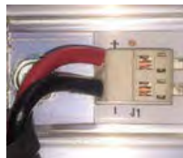
Figure(6) Observe correct polarity when connecting LED power delivery wires
